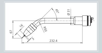
The TBi RoboMIG welding torch RM 50W has a very rugged design with a stainless steel outer tube. Therefore, the factory set TCP will neither be changed by thermal stresses during welding nor collisions.
