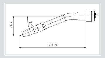
The TBi RoboMIG welding torch RM 60W has a very rugged design with a stainless steel outer tube. Therefore, the factory-set TCP will neither be changed by thermal stresses during welding nor collisions.
